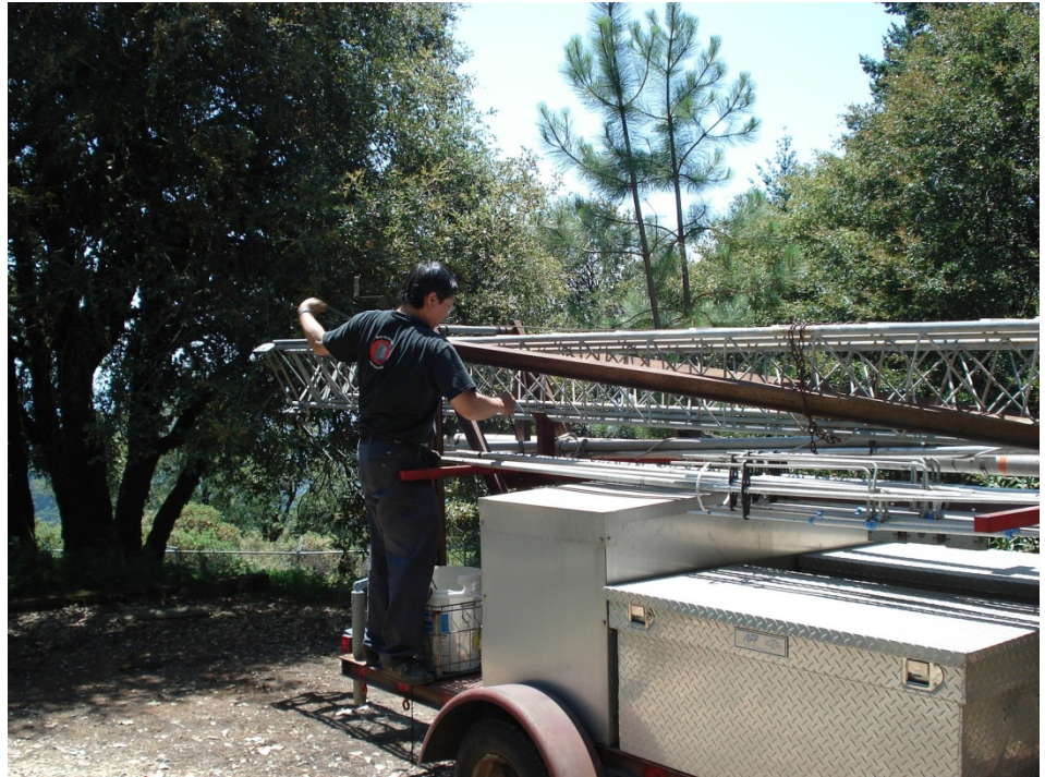
Yin Shih, N9YS, begins deploying the 65' tower mounted to a trailer used to elevate HF antennas.
